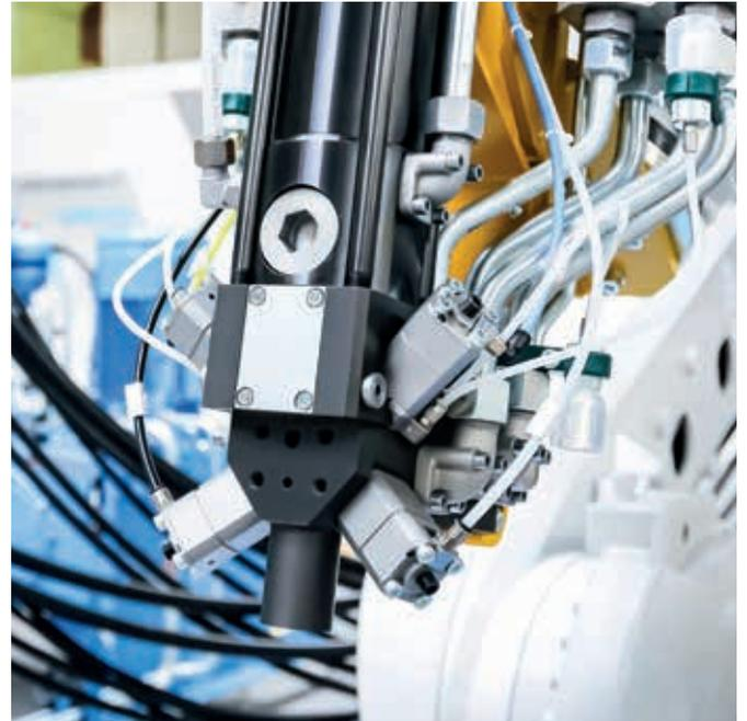
*A perfect pairing for diverse applications in the automotive industry: Four-component mixheads with hermetically sealed FLEXJET GL injectors.*
