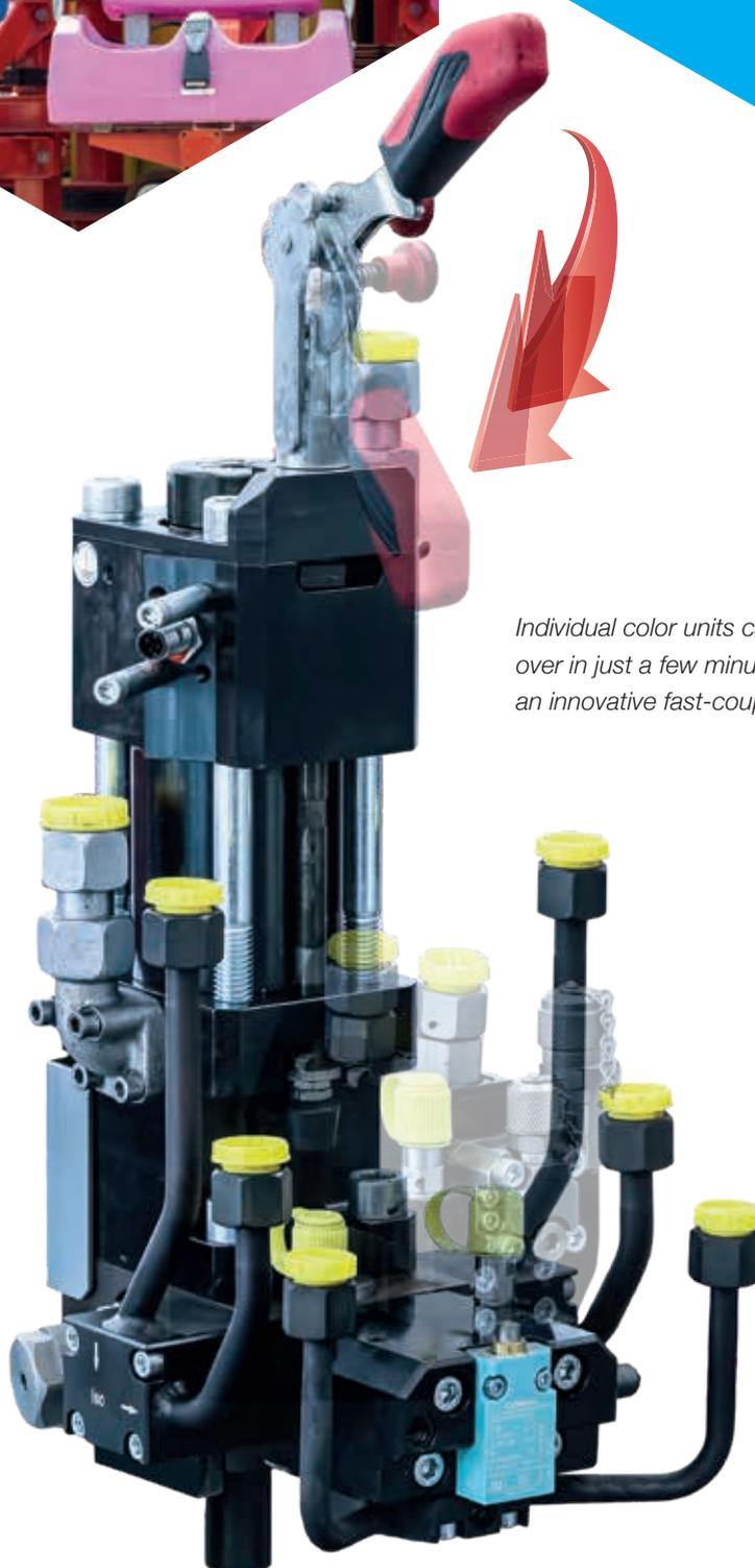
Individual color units can be swapped over in just a few minutes using an innovative fast-coupling system.
