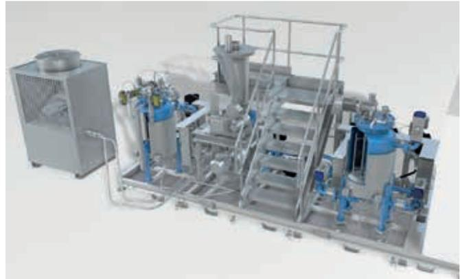
*The ECOFILLER PLUS is the first product from the new Environmental Technologies product line and allows cuttings and material waste from production to be recycled.*
