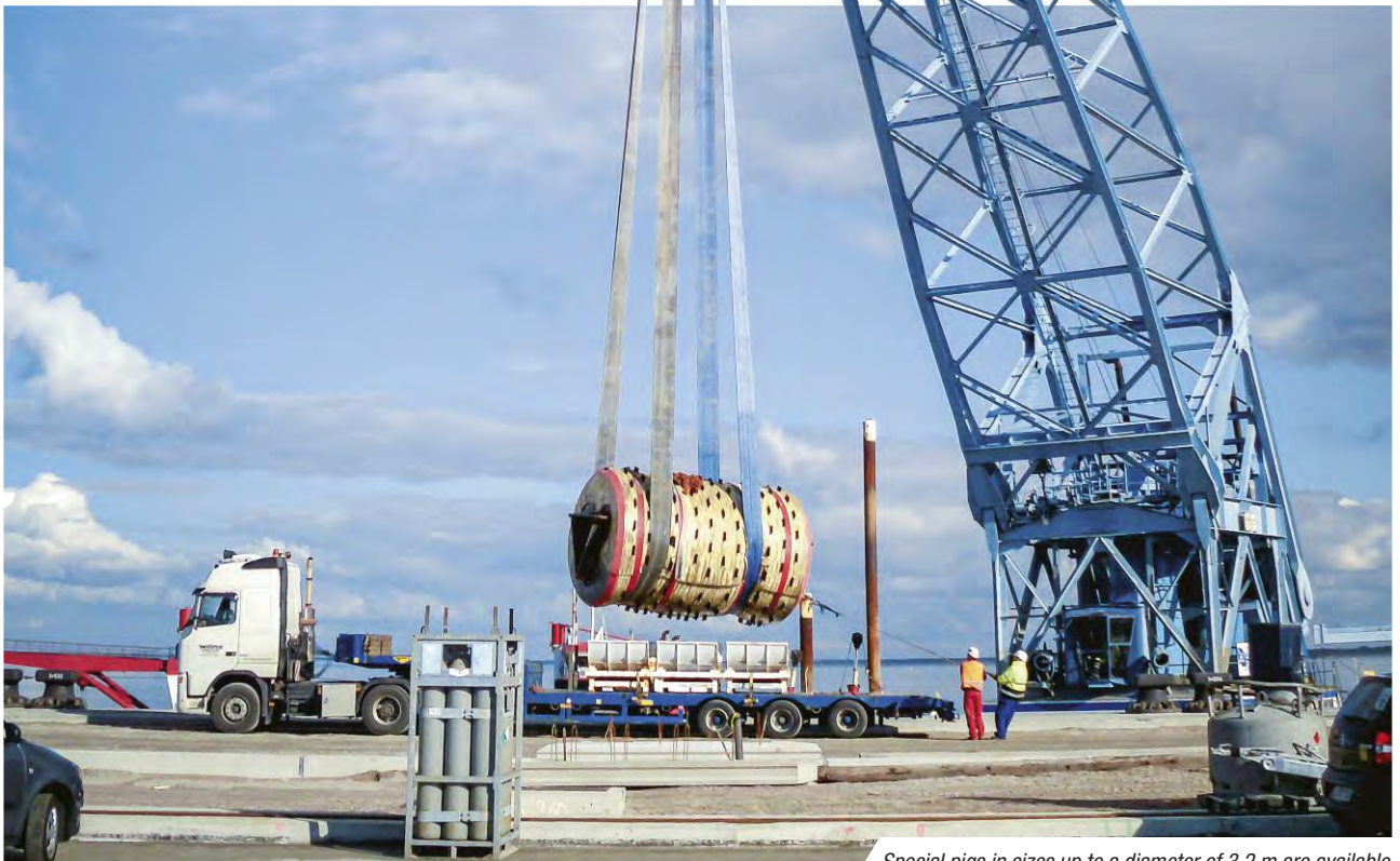
Special pigs in sizes up to a diameter of 3.2 m are available
