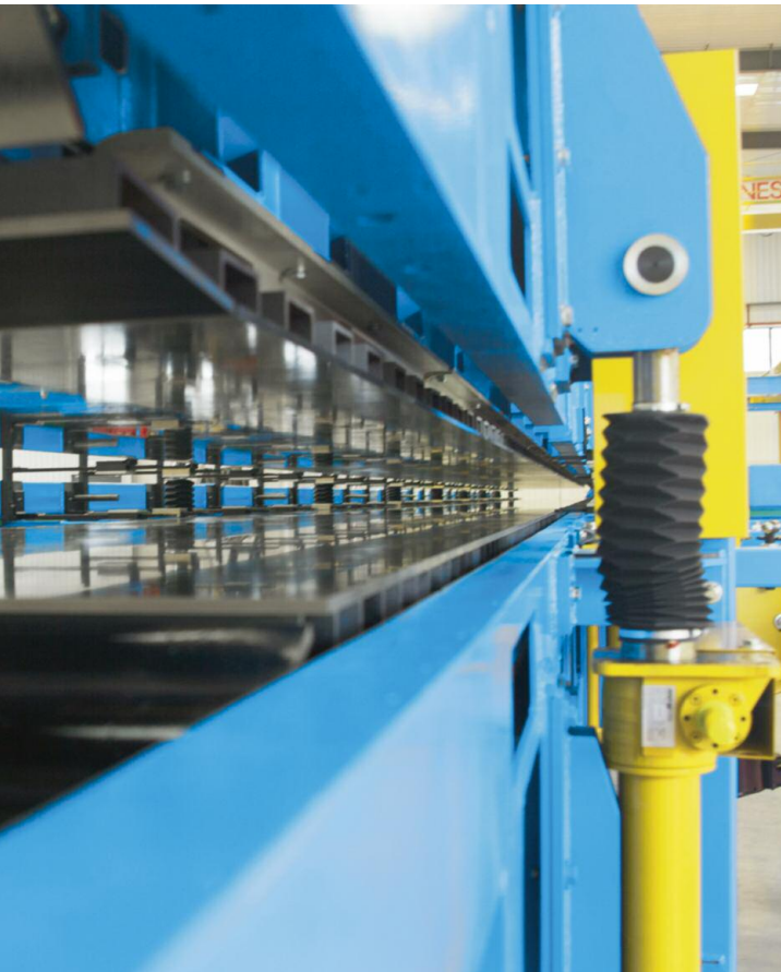
Production quality without any compromise: double plate conveyor from HMS' production facility
