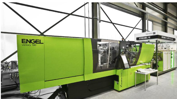
Injection moulding and the HP-RTM process: combined production unit in the Hennecke TECHCENTER
